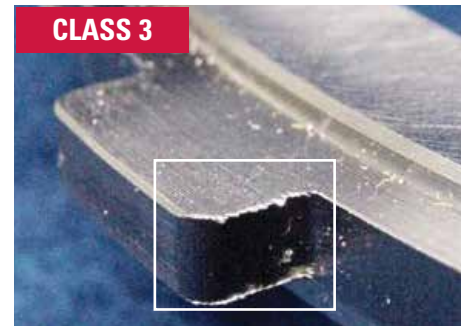
Burrs in this group are well-attached, but relatively small in size. Despite their size, significant mechanical energy must be applied to remove them.
