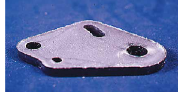
Blanked steel part before deburring.
