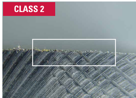
Feather burrs are readily visible without magnification and are characterized by extremely thin roots. They can be removed with a tip of a pencil.
