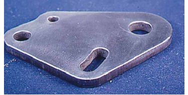
Blanked steel part after deburring.
