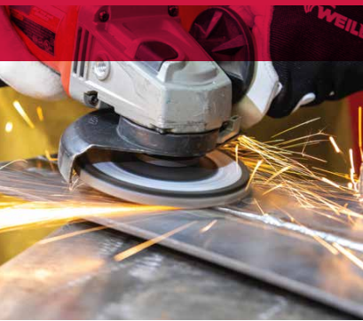
Tiger X flap disc blending a weld on a flat surface.
