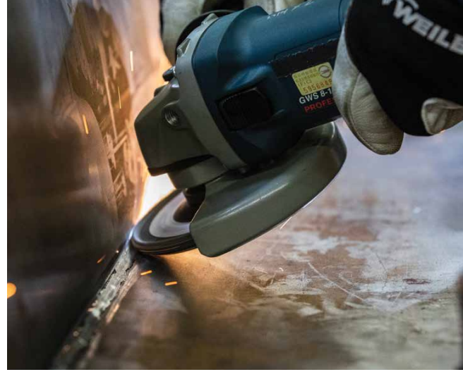
The curved flap design provides optimal contact when grinding fillet welds.
