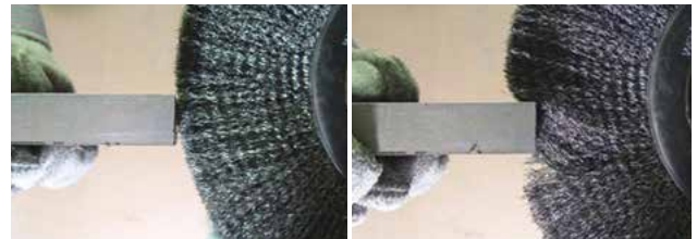
Correct Wire Tips Doing the Work
