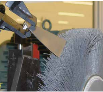
Deburring the tip of a turbine blade.
