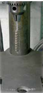
Correct Mounting in Chuck
