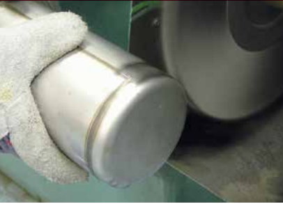
Removing heat discoloration from a stainless steel canister.
