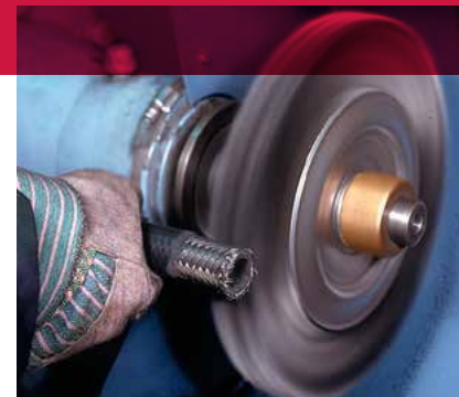
Removing rubber coating from a hydraulic hose.
