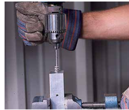
Crosshole deburring an aluminum manifold.
