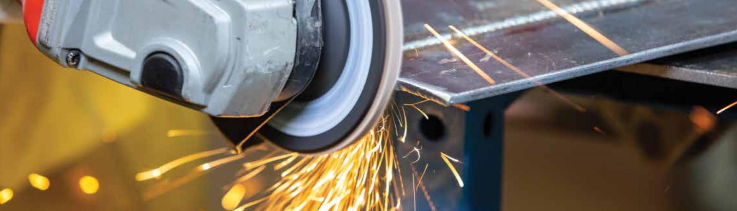
Tiger Paw grinding the edge of a torch-cut steel plate.
