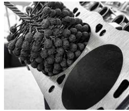
Engine cylinder head honing.
