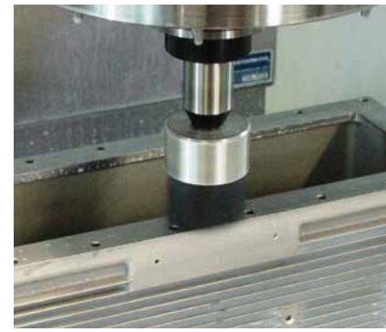
Deburring the machined face of an aluminum component.
