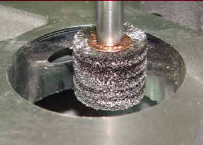
Deburring intersecting oil passages in an engine block.
