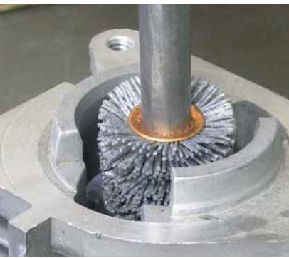
Deburring internal bores of a cylinder head.
