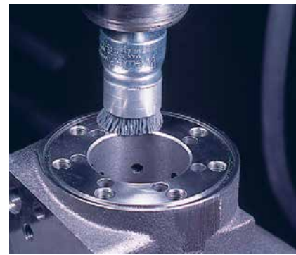
Blending tool marks on a hydraulic component.
