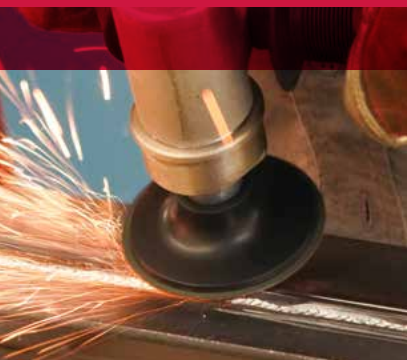
Blending disc smoothing weld seams.
