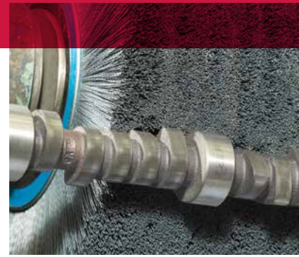
Deburring a camshaft with a Nylox wheel.
